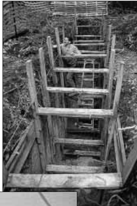
Large pit, excavated to obtain small cores for K_s measurements at the Black Spur site.
