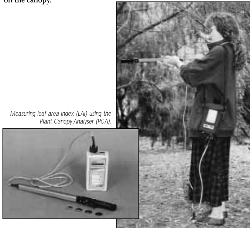
Figure 14: Field of view of the LICOR LAI-2000 Plant Canopy Analyser (PCA). In our study we included data for the field between 0 and 53° only.
