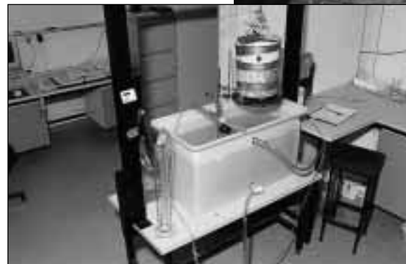
Laboratory apparatus used to determine the K_s of large cores.
