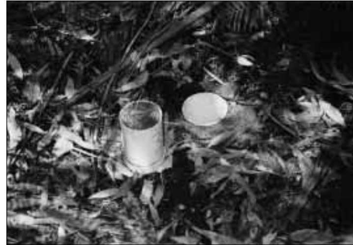
Microlysimeter and access sleeve, used for measuring soil and litter evaporation.
