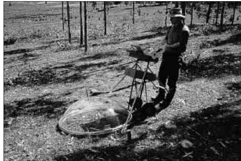
The humidity dome method for measuring soil and litter evaporation.
