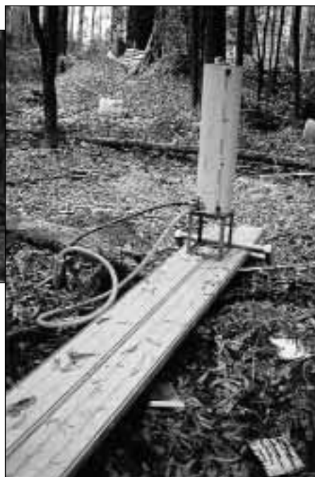
Field measurement of K_s using the borehole permeameter method.
